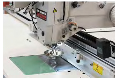
Well-designed machine with gear belt transmission of the sewing carriage for smooth, controlled, operation.
