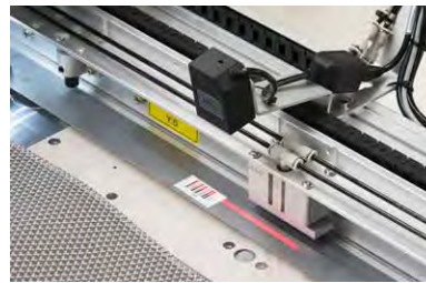
Tooling recognition (bar code) with automatic pattern selection
