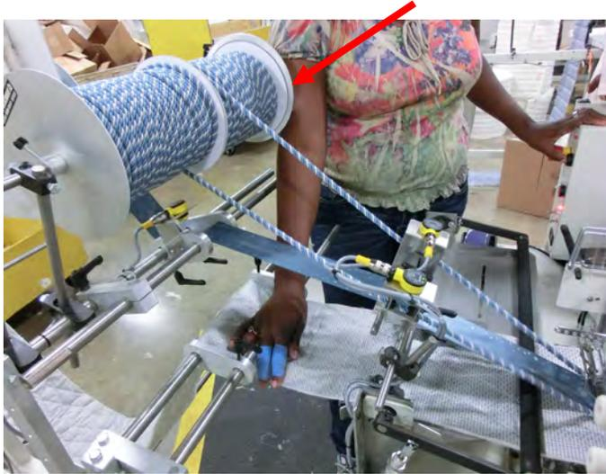
When you get down to the last few layers of the cord it starts to really knot up. We recommend stopping the machine at this time and unroll the rest of the cord from the spools. This will help eliminate the excessive knotting.
