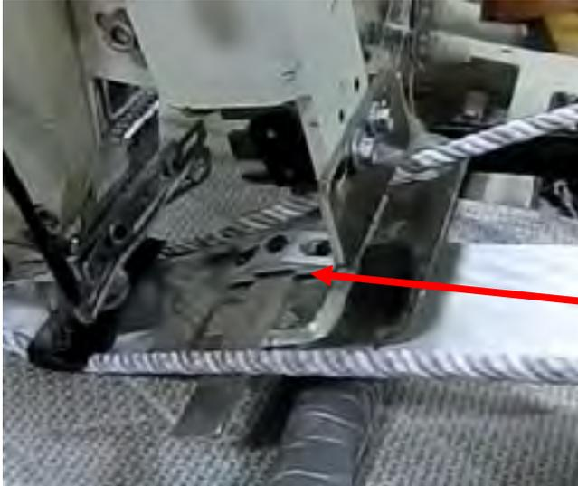
When inserting new tape, cut the tape end to a long point and insert into tube under the old tape end. With a little feeding help, it should sew through with the manual pedal.
