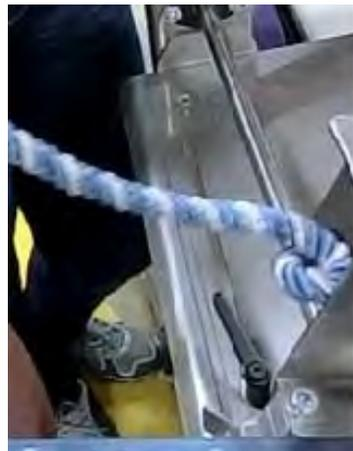
We removed the stainless steel eyelet plate from the top of the tape guide to make it a little easier to insert new cord. It also gives the cord more wiggle room without trapping knots and causing jams. It is necessary to add washers so the screws will tighten properly.
